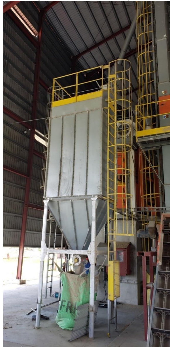
<Figure 12: Dust Collector System>
