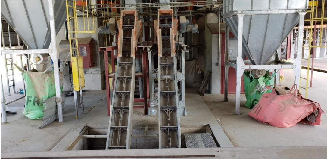
<Figure 9: Chain / Drag Conveyance System>
