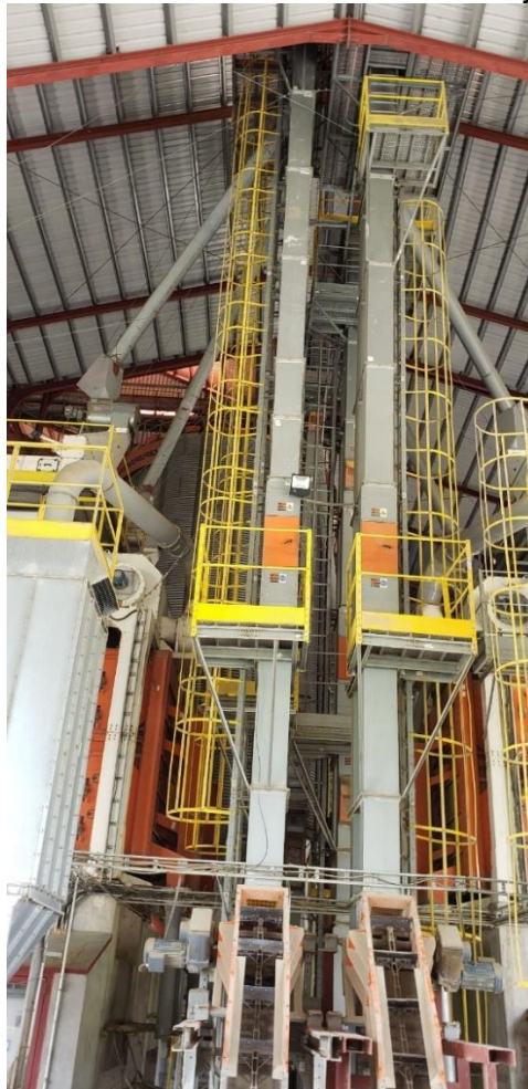
<Figure 10: Carrier Bucket Grain Elevator System>
