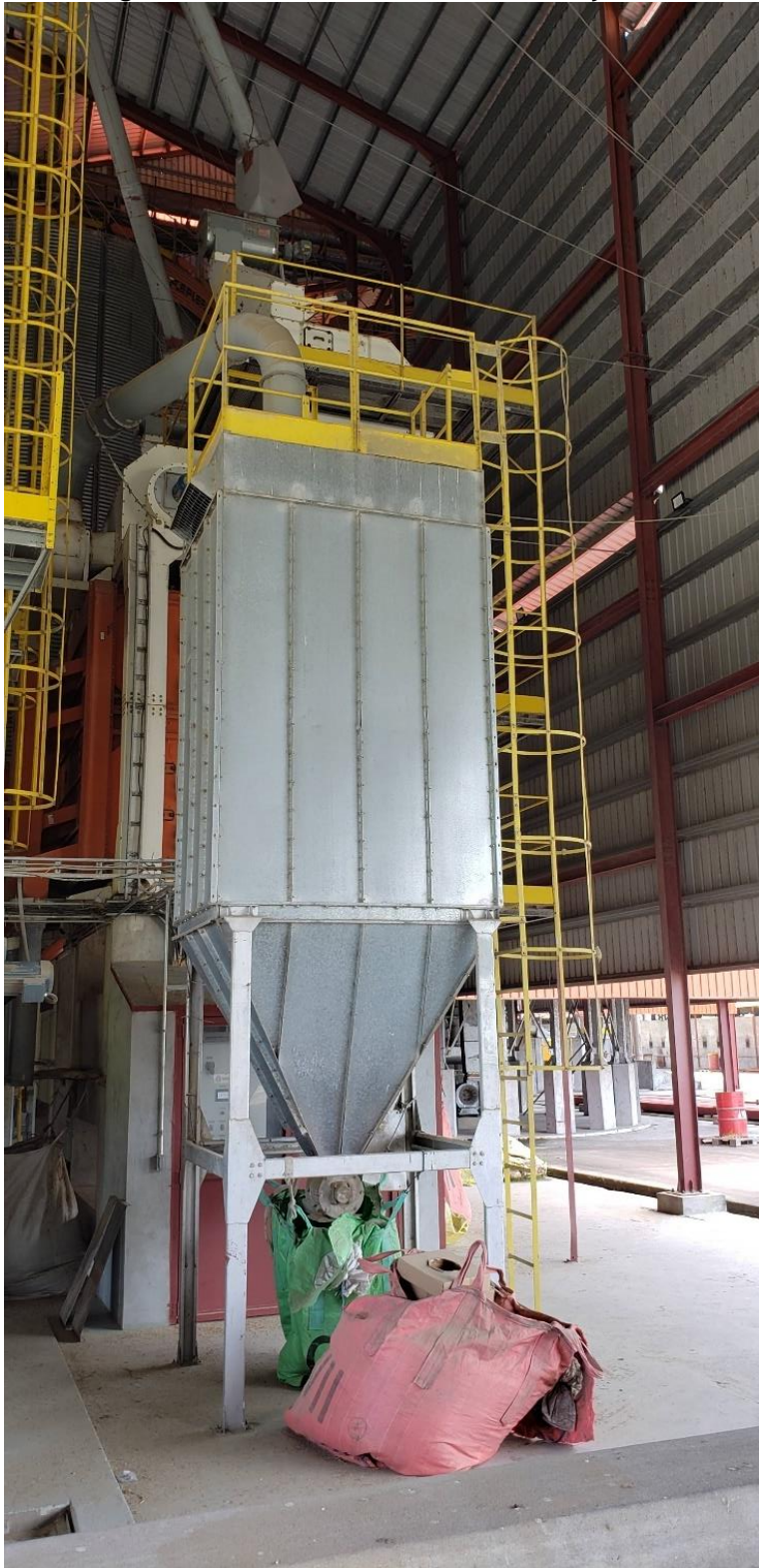
<Figure 42: After Filter Dust Collection Systems>
