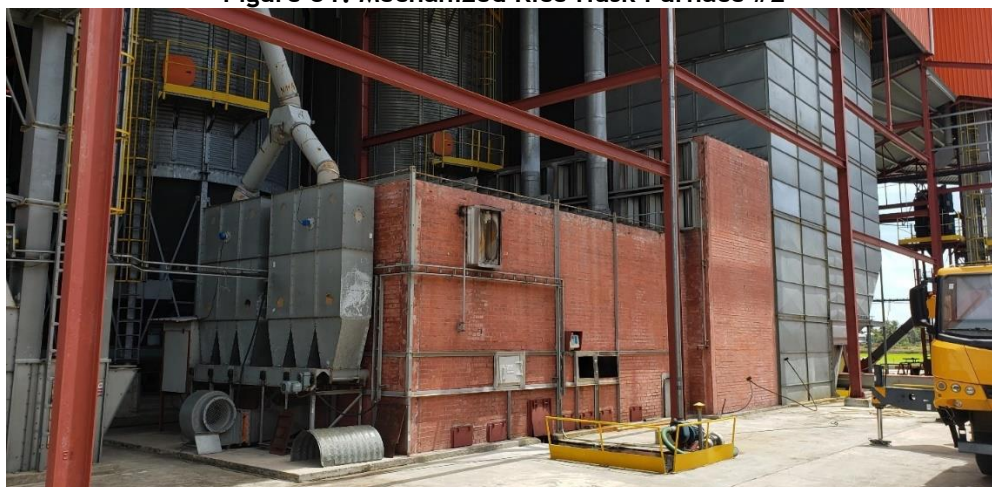
<Figure 31: Mechanized Rice Husk Furnace #2>
