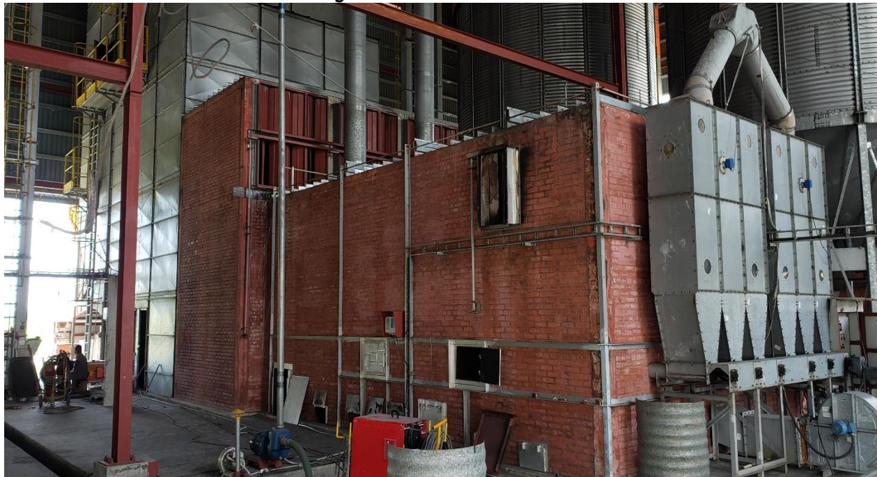
<Figure 14: Biomass Furnace>
