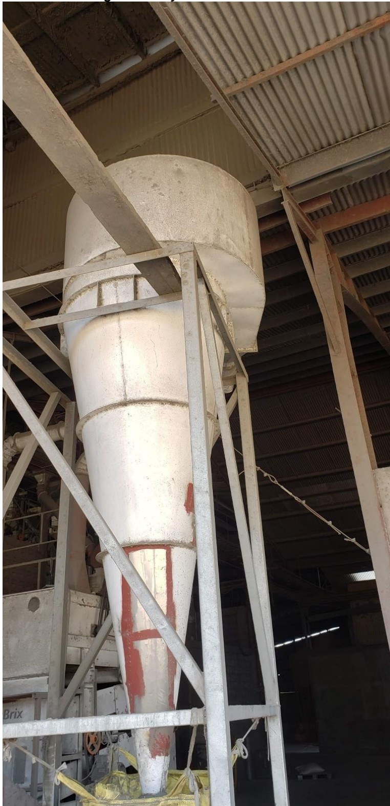
<Figure 45: Cyclone Dust Collector>
